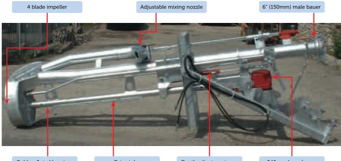
Rubber fluted bearing, slurry lubricated
