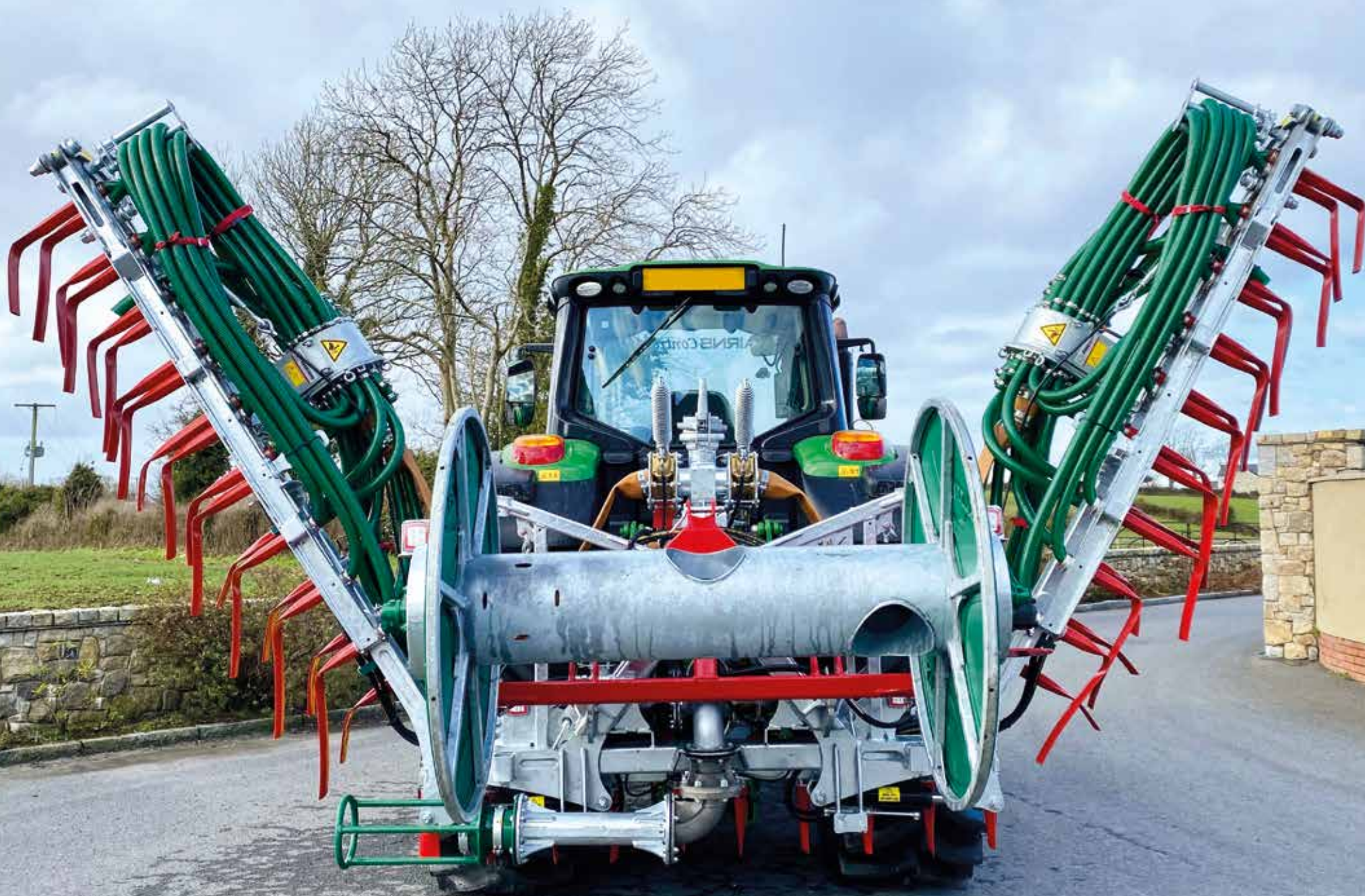
800m reeler mounted on 12m dribble bar
