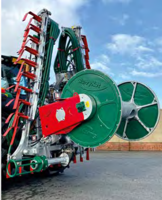
800m reelers front & rear – 1600 metre hose capacity
