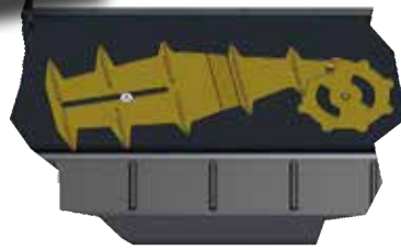
Hydraulic agitator system to prevent bridging
