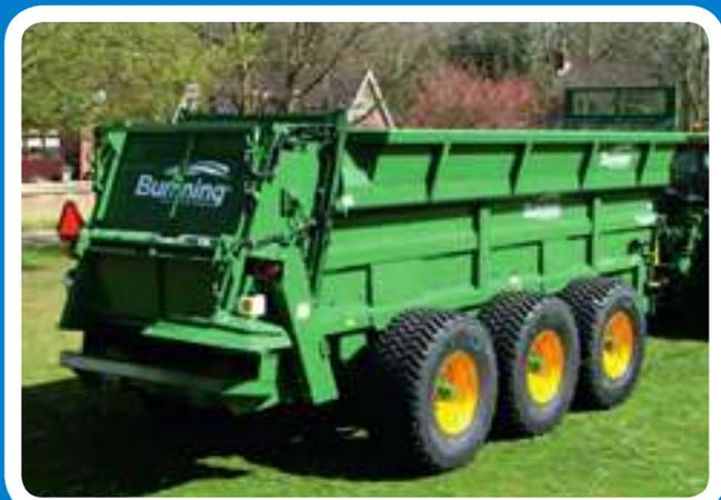
**LOWLANDER WIDEBODY 380 HD HBD** with guillotine slurry door, border deflector and 650/65 R30.5 Michelin tyres, weigh cells and auto rate control.
