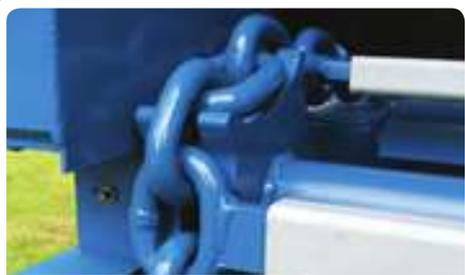
Grade 80, 20mm heavy duty chains are drawn by high tensile sprockets. Sprockets are fitted to the front floor shaft as well as the driven rear shaft, ensuring perfect alignment and timing of the chains, which, in turn makes for a more reliable floor drive. Each chain has a 50 tonne breaking certificate.
