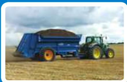
**LOWLANDER 150** with detachable spinner deck, weigh cells, bolt on extension sides, guillotine slurry door and sprung drawbar.
