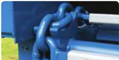
Grade 80, 20mm heavy duty chains are drawn by high tensile sprockets. Sprockets are fitted to the front floor shaft as well as the driven rear shaft, ensuring perfect alignment and timing of the chains, which in turn makes for a more reliable floor drive. Each chain has a 50 tonne breaking load certificate.
