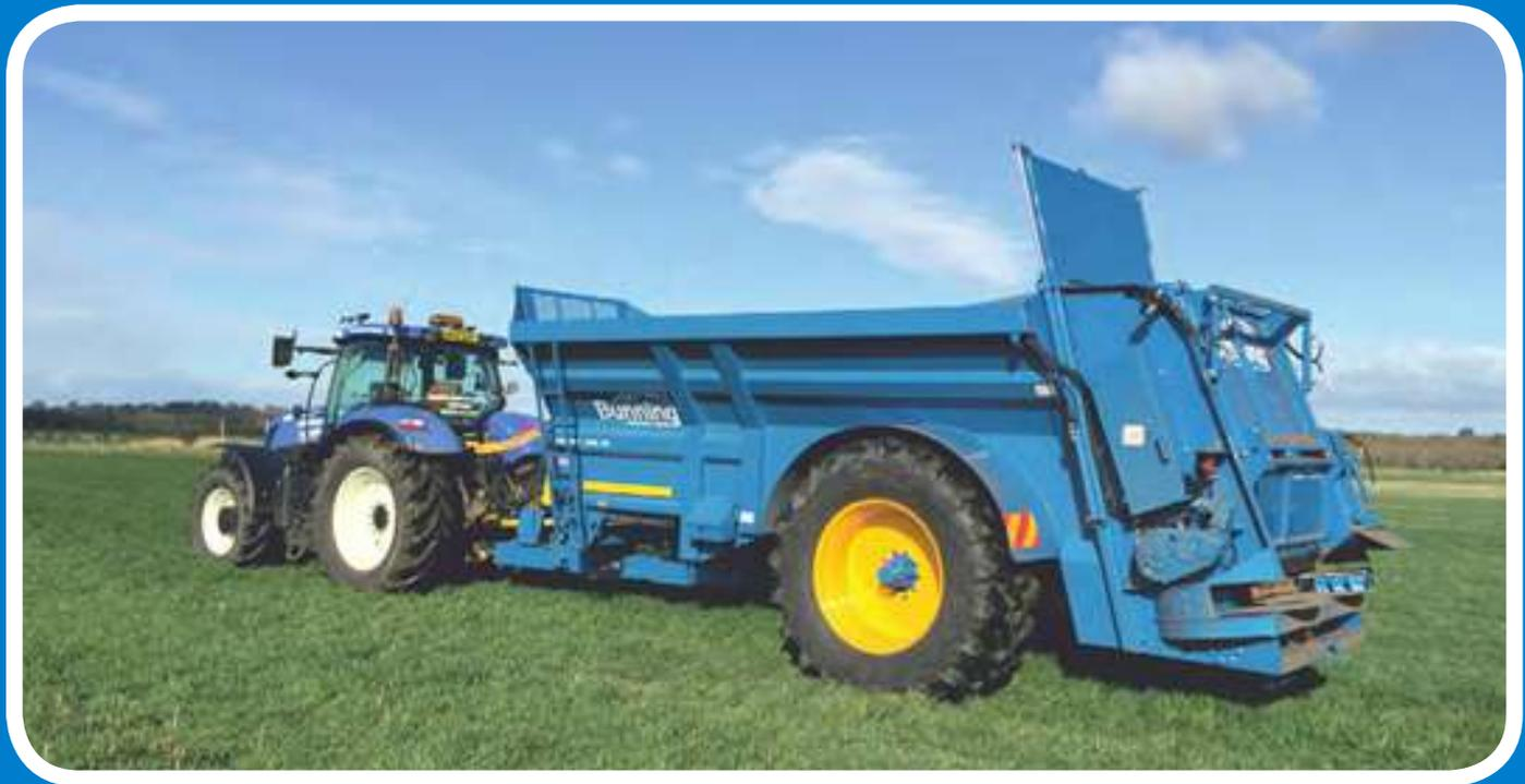
**LOWLANDER 175 HEAVY DUTY HBD** with mudguards, guillotine slurry door, weigh cells and auto rate control, sprung drawbar.
