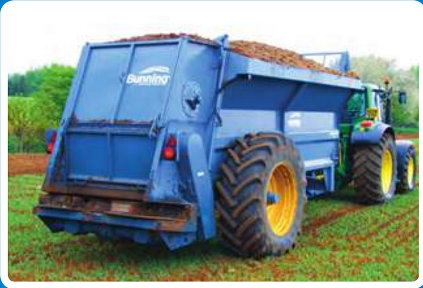
As a dedicated factory build Lowlander spreaders from the 105 Mk4 through to the Widebody 380HD are available with 2 horizontal beaters for processing material onto 2 large diameter spinning discs. Drop on point of material onto the discs and disc blade angles are adjustable for maintaining accurate spread patterns.
