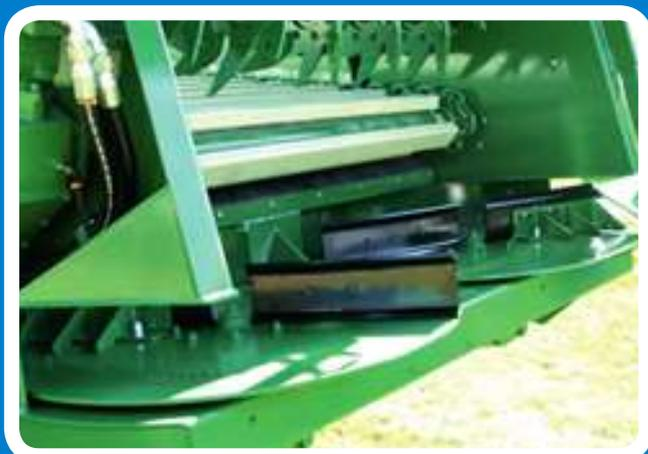
**LOWLANDER WIDEBODY HBD** 2 x 10mm x 1100mm diameter spinning discs with adjustable hardened boron blades.
