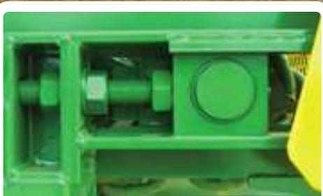
A robust, simple and reliable floor tensioning system ensures floor chain tension can be easily adjusted in order to be kept to its optimum setting.
