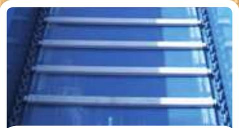
Full width box floor slats clear the whole floor ensuring materials have no chance of bridging in the middle, a problem sometimes encountered with multi chain and slat floor systems.
