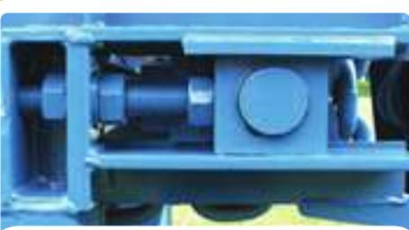
A robust, simple and reliable floor tensioning system ensures floor chain tension can be easily adjusted in order to be kept to its optimum setting. Floor chains are visible from the exterior of the machine making it easy to judge when tensioning is required.
