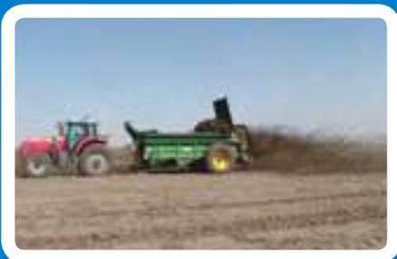
**LOWLANDER WIDEBODY 180 TVA** with guillotine slurry door, 280mm bolt on flared extension sides, sprung drawbar.
