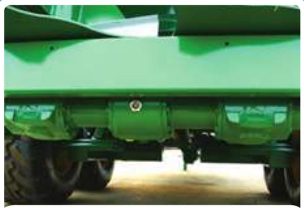
The robust one piece gearbox houses internal gear sets unique to Bunnings in order to ensure that auger speeds are optimised to achieve excellent spread patterns. They are large in diameter with 54mm output shafts manufactured from heat treated steel. The precision machined castings ensure perfect alignment of all the driveline components.
