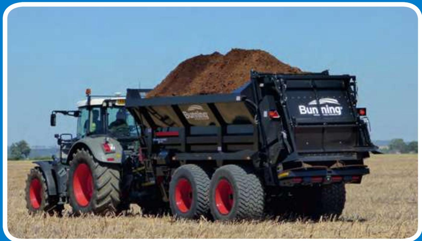
**LOWLANDER WIDEBODY 230 HBD** with built in flared extension sides, 710/50 R30.5 tyres, slurry door, border deflector, steering rear axle and Isobus weigh cell system.
