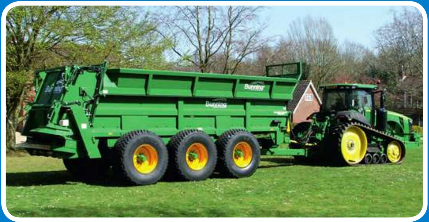
**LOWLANDER WIDEBODY 380 HD HBD** with guillotine slurry door, border deflector and 650/65 R30.5 Michelin tyres, weigh cells and auto rate control.
