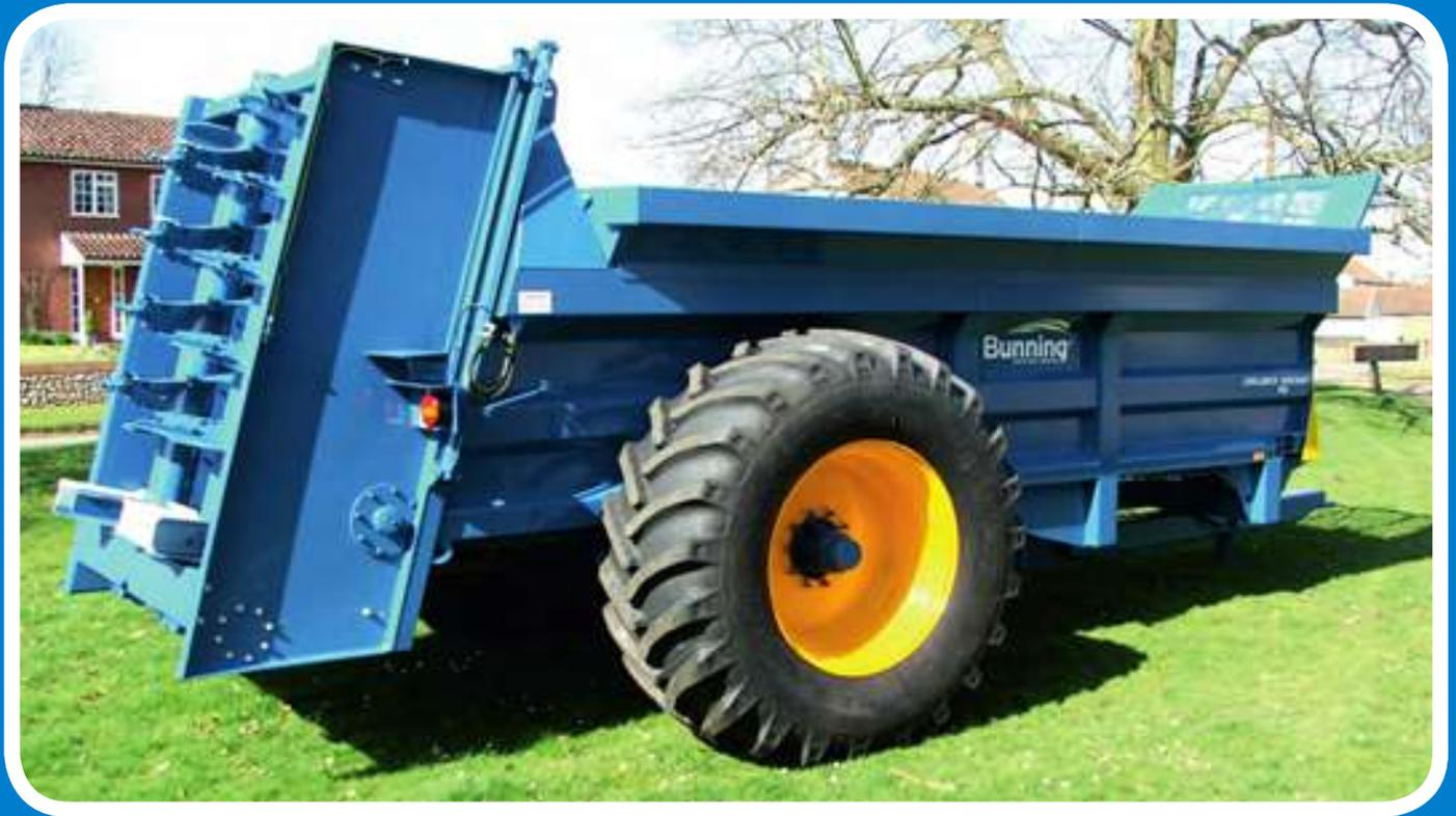
**180 WIDEBODY** with 710/70 R38 tyres, 280mm bolt-on extension sides and sprung drawbar.
