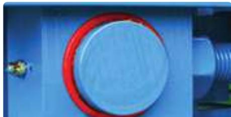
60mm high tensile floor drive shafts rotate through polyester re-inforced composite bushes that contain a solid graphite filler. Chosen for their high load applications in a variety of environments they are greasable, further extending their life.
