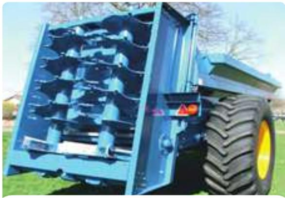
Twin 870mm diameter dynamically balanced vertical augers have flights laser cut from heat treated boron steel to improve strength and service life.
