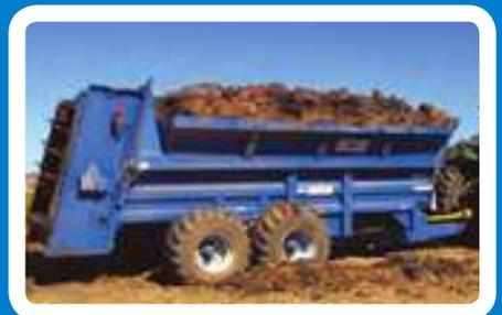
**Lowlander 230 WIDEBODY** with bolt-on flared extension sides, sprung drawbar and guillotine slurry door.
