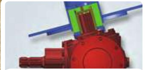
Especially developed to reduce shock loads to the auger drive gearbox, the rubber cushion arrangement located between the output shaft of the auger gearbox and the base of the auger contributes to the reliability and longevity of the machine. Rubber cushion highlighted in green.
