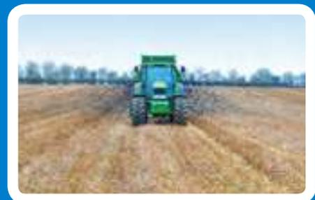
**LOWLANDER 150 HD** sludge cake build with flared body, guillotine slurry door and 710/70 R38 tyres, spreading bio solids.
