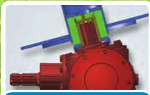
Especially developed to reduce shock loads to the auger drive gearbox, the rubber cushion arrangement located between the output shaft of the auger gearbox and the base of the auger contributes to the reliability and longevity of the machine.
