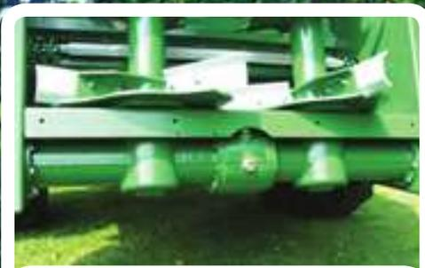
The robust one piece gearbox houses internal gear sets unique to Bunnings in order to ensure that auger speeds are optimised to achieve excellent spread patterns. They are large in diameter with 54mm output shafts manufactured from heat treated steel. The precision machined castings ensure perfect alignment of all the driveline components.
