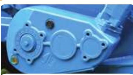
The 800 series floor drive gearbox is fitted to all the Heavy Duty models. It is hydraulically driven to ensure an even feed of material to the spreading mechanism at all times. With a reverse feature, any foreign object too large to pass through the beaters can be easily removed. An adjustable crossline relief valve also delivers additional protection.
