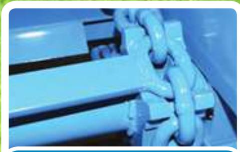
Grade 80, 16mm heavy duty chains are drawn by high tensile sprockets. Sprockets are fitted to the front floor shaft as well as the driven rear shaft, ensuring perfect alignment and timing of the chains, which in turn makes for a more reliable floor drive. Each chain has a 32 tonne breaking strain certificate.
