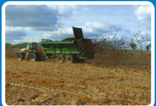
**LOWLANDER 230 WIDEBODY** sludge cake build with built-in flared extension sides, wheels under body, and guillotine slurry door.
