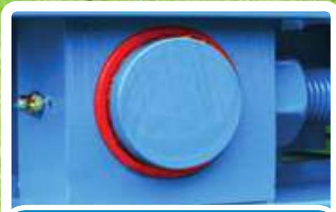
50mm high tensile floor drive shafts rotate through polyester re-inforced composite bushes that contain a solid graphite filler. Chosen for their high load applications in a variety of environments they are greasable, further extending their life.
