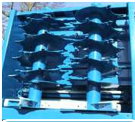
Twin 870mm diameter dynamically balanced vertical augers have flights laser cut from heat treated boron steel to improve strength and service life.
