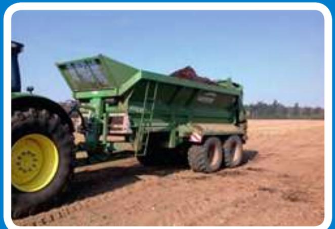
**LOWLANDER WIDEBODY 230 HBD** with built in flared extension sides, guillotine slurry door, sprung drawbar, weigh cells and 600/55 R26.5 tyres.
