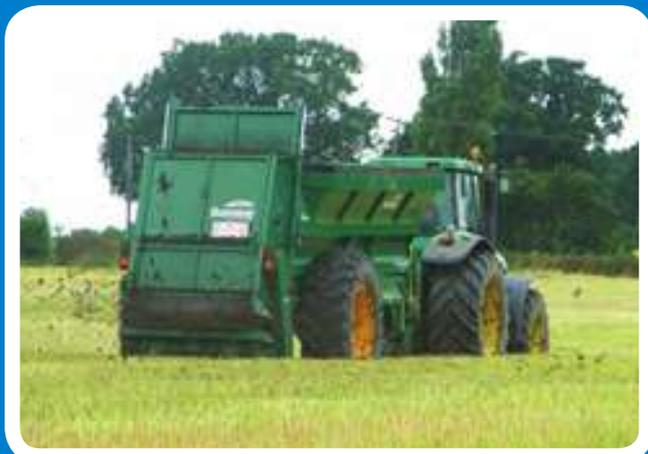
**LOWLANDER 180 WIDEBODY HBD** with 2 horizontal beaters & spinning discs, weigh cells, bolt on flared extension sides and 710/70 R38 tyres.
