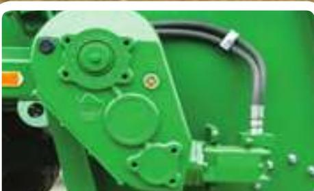
The 800 series floor drive gearbox is fitted to all models within the range. It is hydraulically driven to ensure an even feed of material to the spreading mechanism at all times. With a reverse feature, any foreign object too large to pass through the beaters can be easily removed. An adjustable crossline relief valve also delivers additional protection. The 320 and 380HD models are fitted with 2 floor gearboxes as standard.
