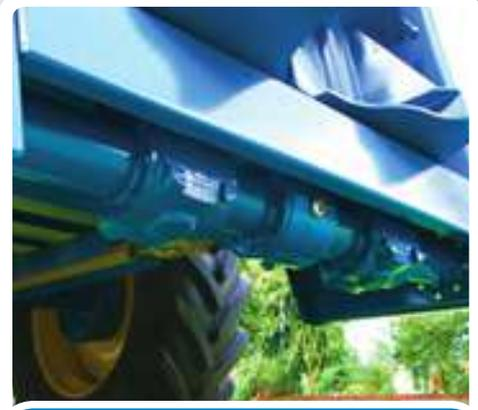
The robust one piece gearbox houses internal gear sets unique to Bunnings in order to ensure that auger speeds are optimised to achieve excellent spread patterns. They are large in diameter with 54mm output shafts manufactured from heat treated steel. The precision machined castings ensure perfect alignment of all the driveline components.
