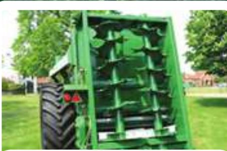
Twin 700mm diameter dynamically balanced vertical augers have flights laser cut from heat treated boron steel to improve strength and service life.
