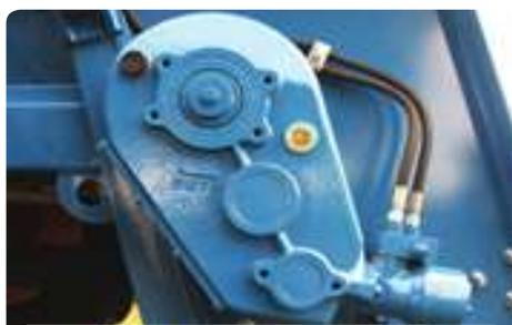
The 500 series floor drive gearbox is fitted to all models with the exception of the Lowlander 60 & 150 (fitted with 350 series & 800 series respectively). It is hydraulically driven to ensure an even feed of material to the spreading mechanism at all times. With a reverse feature, any foreign object too large to pass through the beaters can be easily removed. An adjustable crossline relief valve also delivers additional protection.
