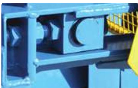
A robust, simple and reliable floor tensioning system ensures floor chain tension can be easily adjusted in order to be kept to its optimum setting. Floor chains are visible from the exterior of the machine making it easy to judge when tensioning is required. Floor shafts are 50mm diameter (60mm on the 150 model), both high tensile.
