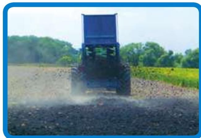
LOWLANDER HD 150 with guillotine slurry door and sprung drawbar.
